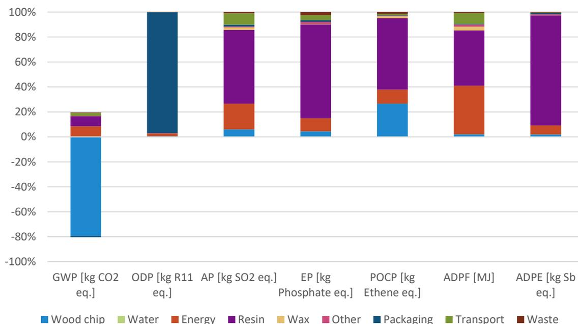
**Figure 3: Contribution from different materials and process steps to the total impact (A1-A4) for the impact categories assessed in this EPD study for MDF manufactured in Cowie**
