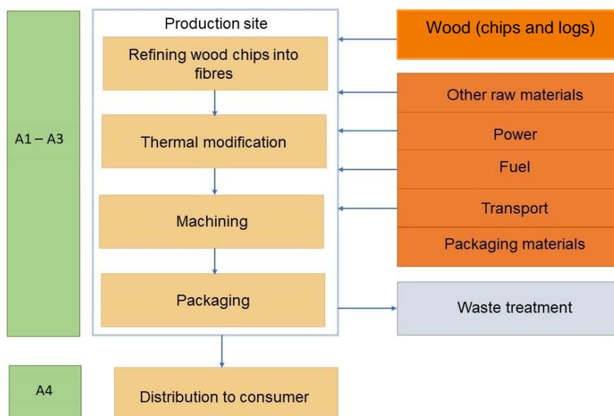
**Figure 2: Process flow diagram showing the production and distribution of Norbord MDF**
